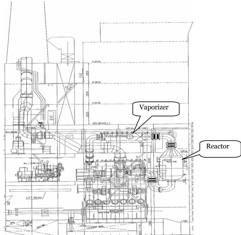
Figure 3: Pre-T/C SCR arrangement in engine room
