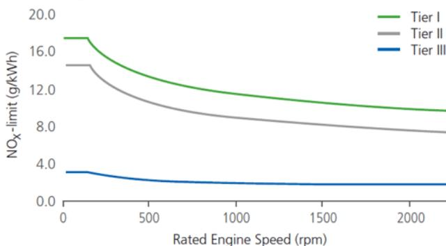
Figure 1: NOx regulations for new engines (source DNV [http://www.dnv.com/industry/maritime/servicessolutions/maritime\\_environment/nox/](http://www.dnv.com/industry/maritime/servicessolutions/maritime_environment/nox/))
